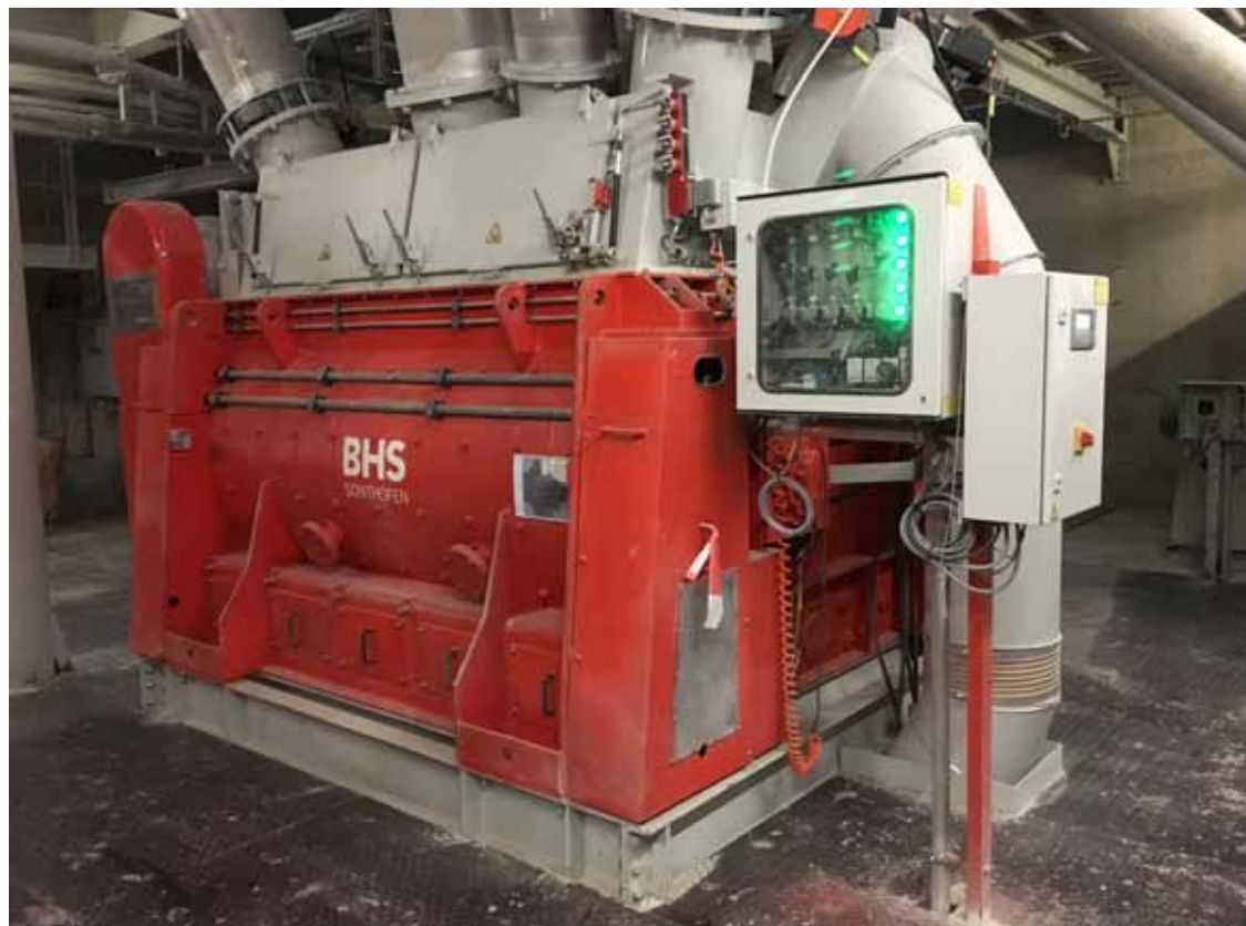
1 BHS dry powder batch mixer of type DMX 4900 at the Wopfing South plant
