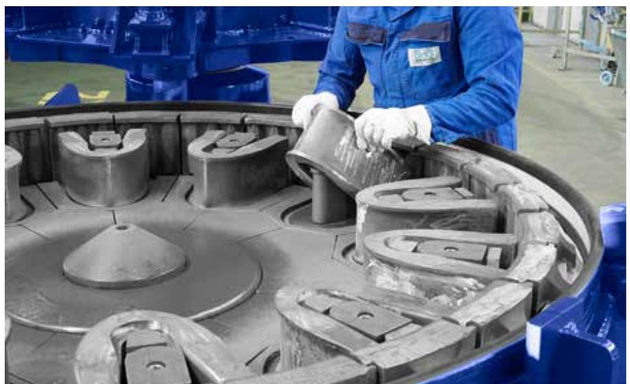
The hammers and the elements of the outer wall are exchanged without tools
