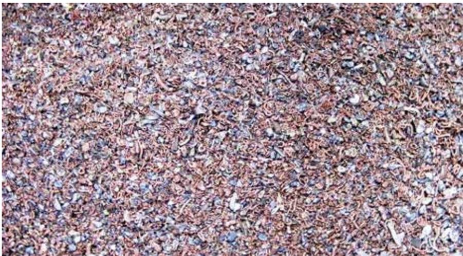
The result: non-magnetic metals with a grain size of 0 - 3 mm
