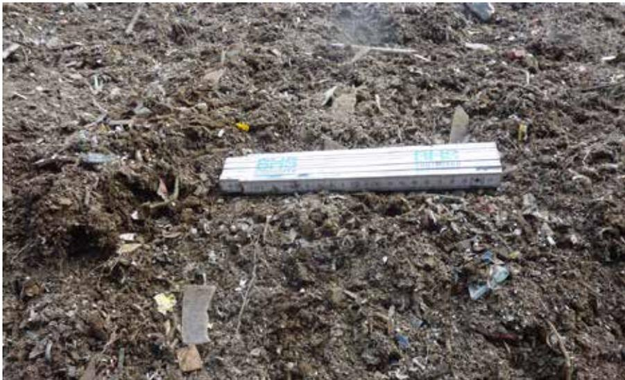
The input material consists of the fine components from coarse shredding
