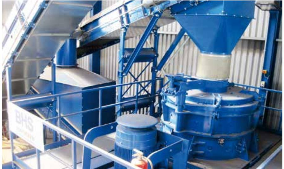
The rotor impact mill of type RPMV in a plant for the fine crushing of shredder waste materials
